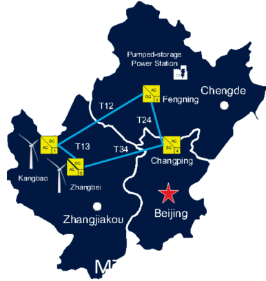
Zhangbei HVDC grid
